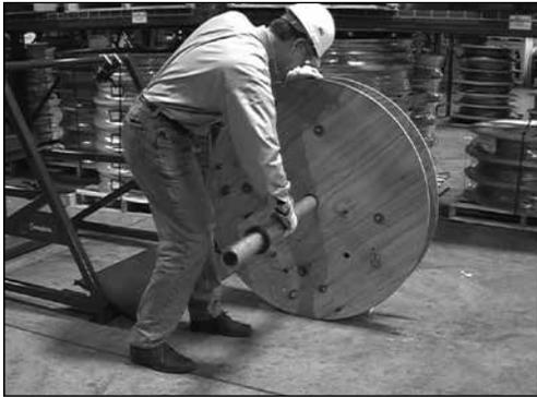
1. Install support spindle through center hole in spool and install collars.
