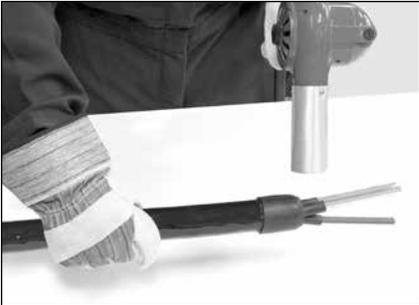
3. Use a heat gun to shrink the boot over the tubing. Move the heat source back and forth over the boot, applying heat evenly. Once the boot has assumed the shape of the tubing, stop applying heat. Further heating will not make the boot shrink any more tightly.
