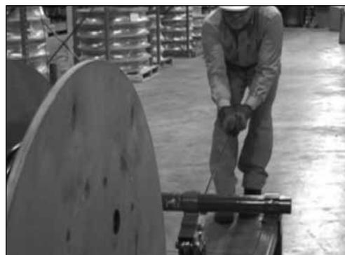
4. Pull tube to create straight section of required length.
