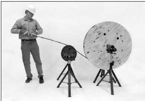
**Method 3:** Use the Swagelok five-roll tube straightener to straighten bare and jacketed tubing in sizes from 1/8 in. to 1/2 in.
