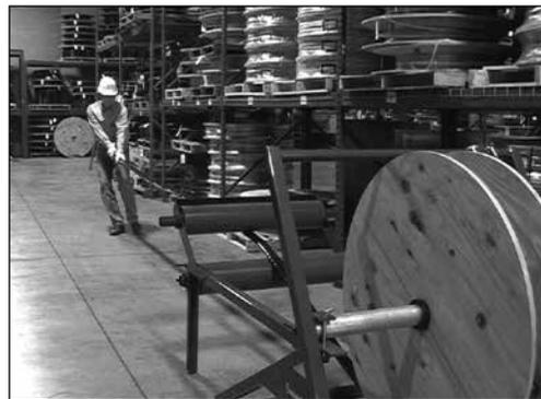
7. Continue to pull tubing through rollers to desired length.
