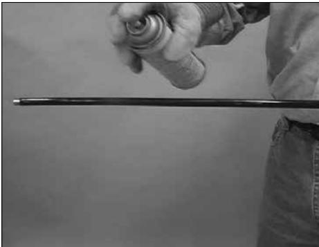
2. Liberally lubricate jacket before bending with silicone spray or light oil to prevent tearing of the jacket.
