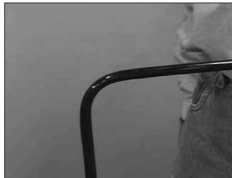
6. After bend is complete, inspect the condition of the bend to make sure jacket is intact.
