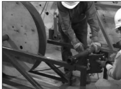
3. Adjust straightener to straighten tube.
