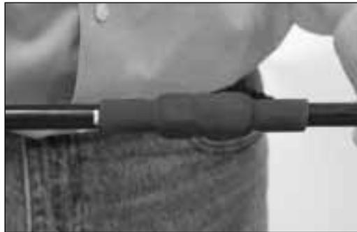
6. When complete the sleeve should be uniform and there should be a small line of adhesive visible between the heat shrink sleeve and the jacket.
