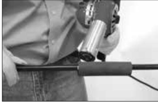
4. Use a heat gun to shrink the sleeve over the tube and fitting. Keep the heat moving so you do not scorch or burn the sleeve or jacket.
