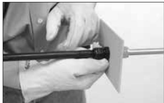
5. A second layer should be applied in the opposite direction of wrapping.
