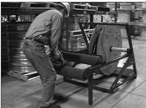
4. Thread tubing between rollers.
