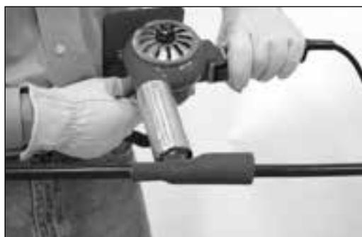
5. Start applying heat at the center of the sleeve and move out to the end. Repeat pattern to seal other end.
