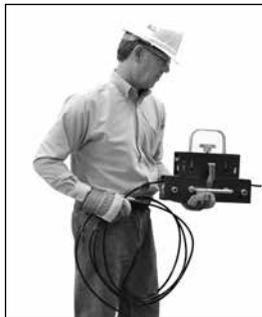
**Method 4:** Mount spool on spool stand with five-roll straightener attachment.
