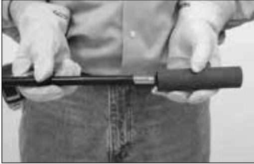
1. Slide the sleeve over the tube before making the connection. Sleeve contains heat-activated adhesive on the inside surface.
