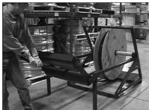
6. With a steady motion, pull tubing through roller assembly.
