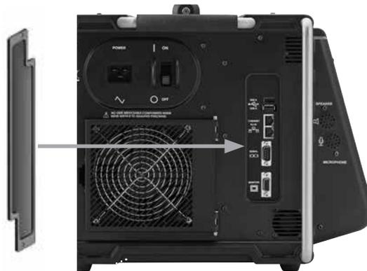
3. Install the new screws and tighten until screws and port cover are flush. Turn screws 1/16 turn past flush.
